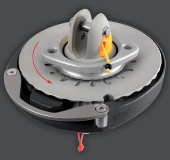
Unlike traditional code sail furling, spinnaker furling starts from the top of the sail. The tack swivel on KSF furler makes sure the furling is safe and does not damage the spinnaker.
