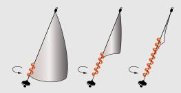
This is the principle of the traditional winding. It owes its name to the torque transmission that happens from the bottom upwards. The sail is secured with a lashing on both ends of the cable; the torsional force is applied to the drum and the textile cable transmits the torque along the cable to the opposite end (at the top); the sail wraps from the bottom to the top.
