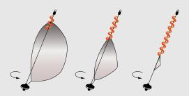
In this case, the tack of the sail is fixed to the specific swiveling drum (free tack): The torsional power applied to the drum is transmitted almost instantly to the swivel at the top and this causes the winding of the sail from the top to the bottom. Once completed the winding, the halyard can be released and the sail can be easily stricken and stowed.
