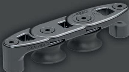
Low friction deck organizer featuring a plain bearing sheave, each component can fit into another and be installed as a curve. The fastening pattern makes it possible to install a KJ2 or KJ3 cam cleat on top of it.
